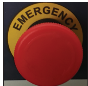
Figure 35 Emergency stop button
