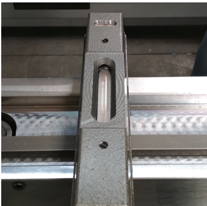
Figure 9 Leveling in transverse and lengthwise directions
