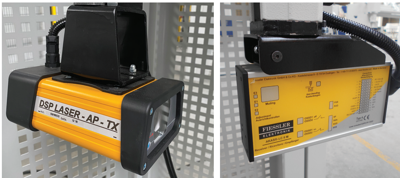
Figure 31 Current laser front security
