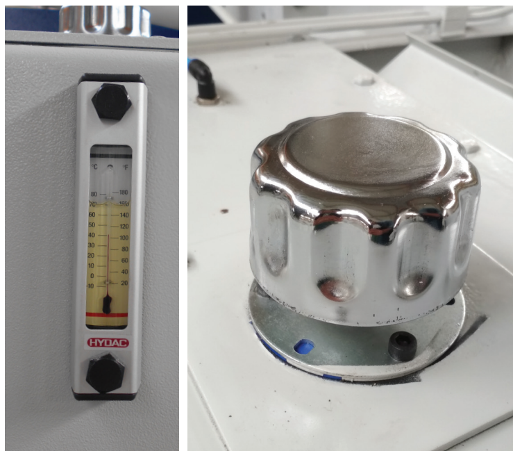
Figure 52 Hydraulic oil gauge and filling cap
