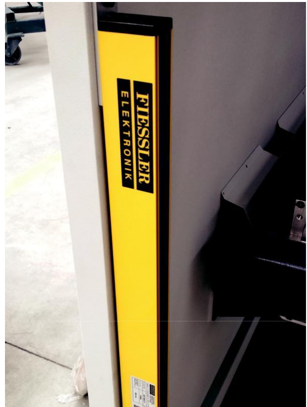
Figure 32 Laser light curtain used for the rear security
