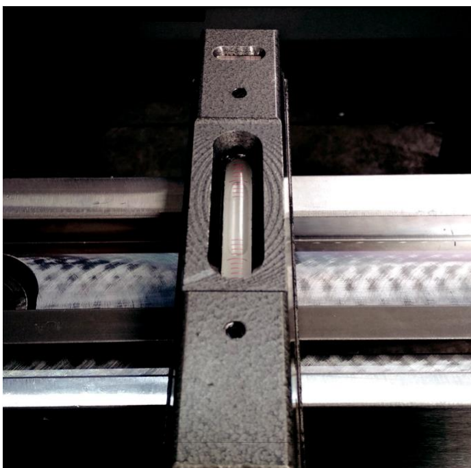
Figure 9 Leveling in transverse and lengthwise directions
