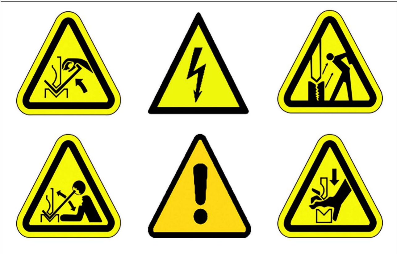
Figure 1 Safety warning signs
